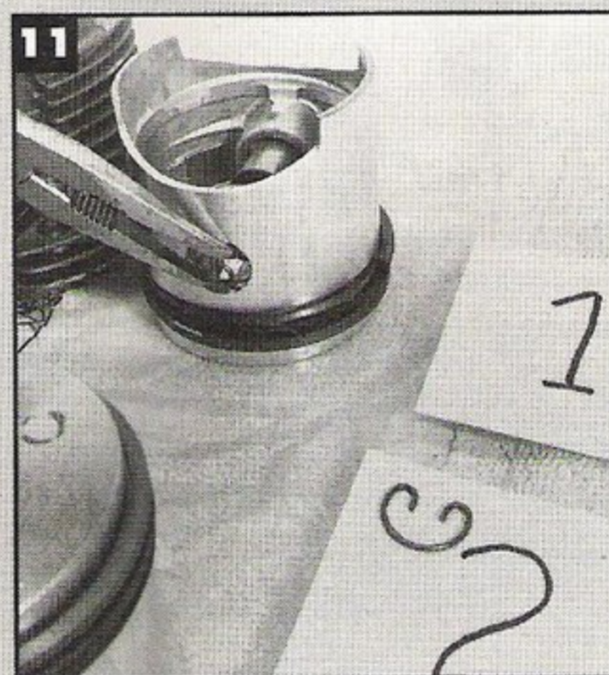
11 - Upon assembly you will be inserting the wrist pins from the outboard ends, so now install a circlip on the inboard side of each piston.
