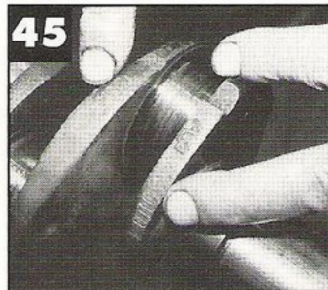
45 - The rod journal also shows excessive abuse and lack of oil. This crankshaft will have to be reground or replaced.
