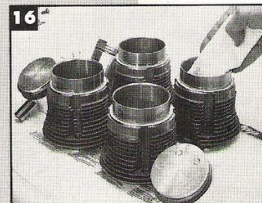
16 - With some clean oil on a clean lint-free cloth, wipe the inside of the barrels thoroughly and you will see some dirt picked up by the cloth even though you cleaned them. This will also leave enough oil on the cylinder bore to prevent scratching the new rings. Leave the rings dry and they will break in properly.
