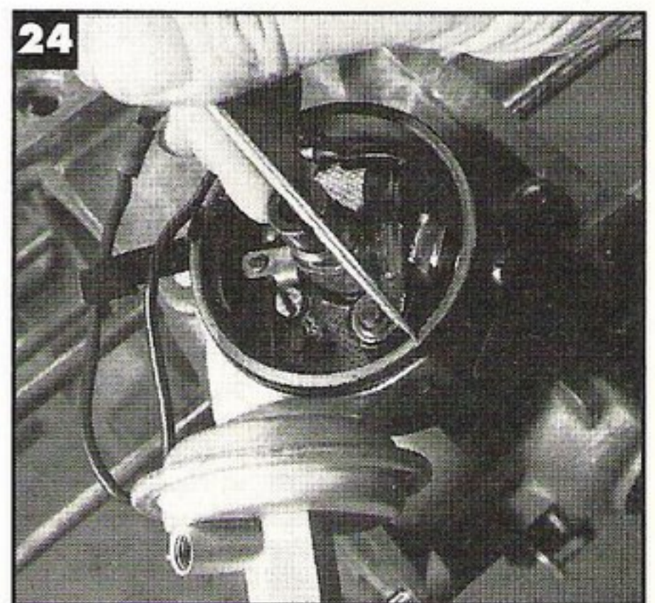
24 - Loosely attach the vacuum chamber to the distributor using a handmade thin cardboard gasket. Tighten the pull rod bracket screw and ground wire lead. Install the rotor and bring it in line with the mark on the edge of the distributor. In this position the points should have just started to open. It is best checked with a test light. If it is impossible to obtain this condition by shifting the vacuum chamber in the mounting screw holes, the length of the pull rod should be altered and the nut readjusted to .138 inches plus or minus .006 inches. Then tighten the screws.
