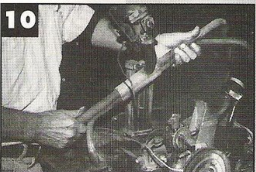
10 - If you took my advice to use a single tool wherever possible, you will have already removed the four nuts that clamp the intake manifold to the cylinder head; now you can just lift off the intake manifold.
