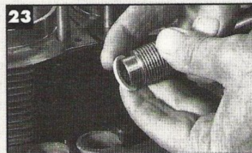
23 - Carefully install all pushrod tube seals by pulling on from one side. Pushing them straight on will at times cause a cut from the sharp edge of the pushrod tube.
