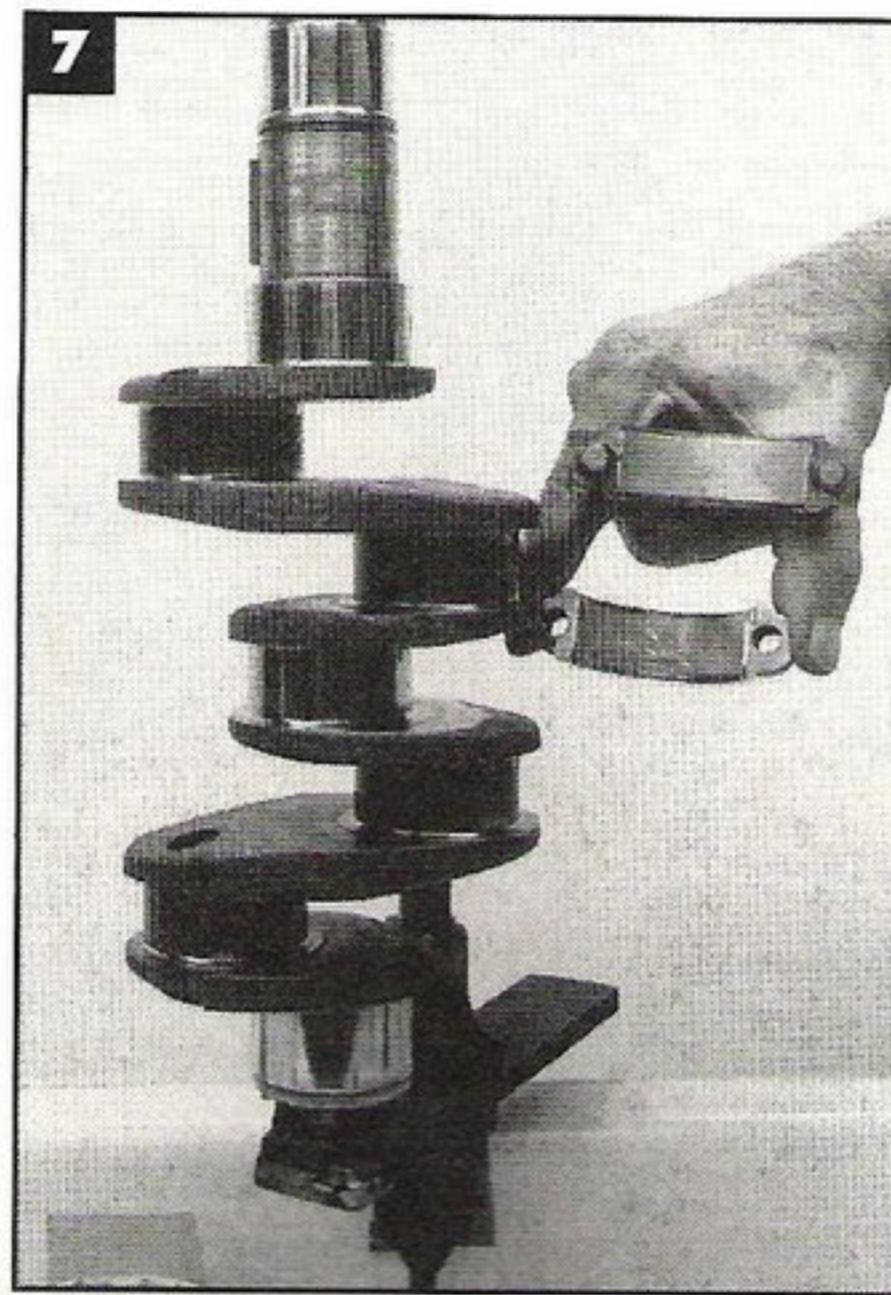
7 - The new .010-inch undersize rod bearings are fitted to the rod and cap, then oiled.
