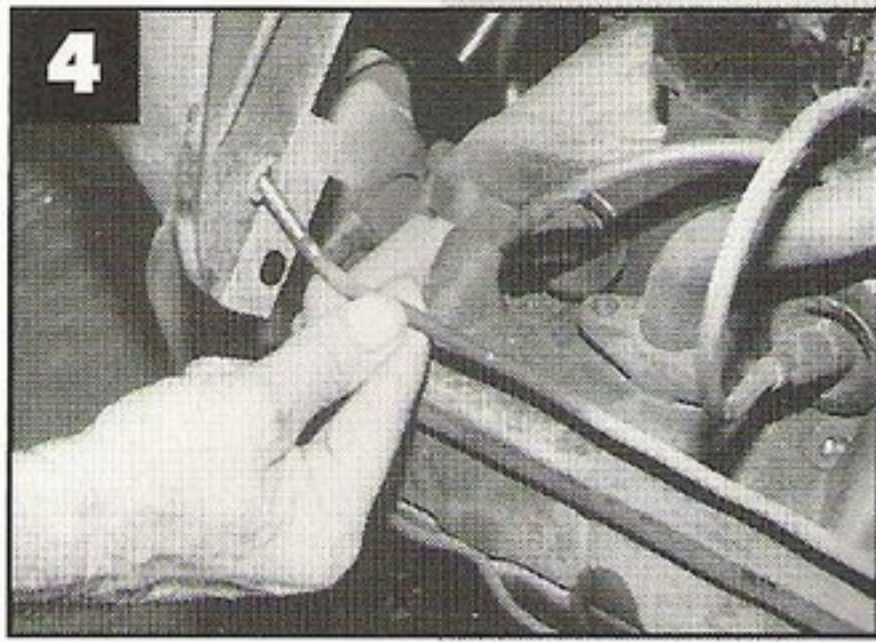
4 - Remove the front sheet metal that seals at the firewall. Note the grommet on the fuel line; when this is worn or missing, the sheet metal will cut into the fuel line. You may need to replace both.
