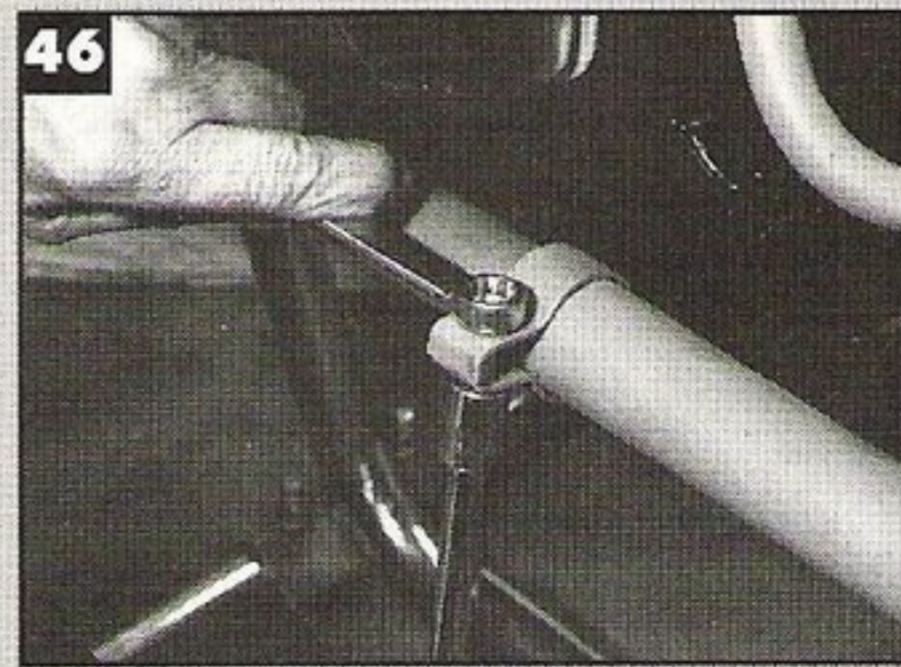
46 - The 36 hp engine doesn't use the later-style asbestos donut gaskets and clamps. It uses a simple slip fit and clamp as shown. Please, no American muffler clamps here as they crush and distort the tubes.
