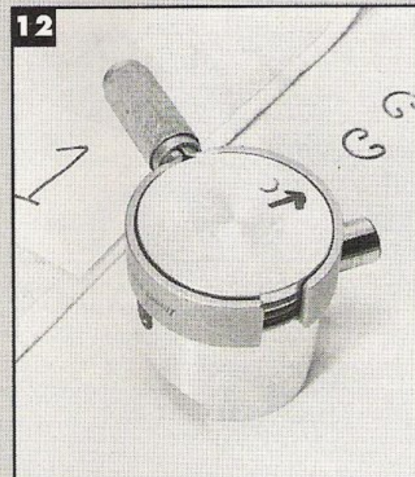
12 - Remember the photo of all the ring gaps lined up and the scorched piston during disassembly? We don't want that to happen so set the lower oil control ring up to the top at the 12 o'clock position, the middle oil scraper ring at 4 o'clock and the top compression ring at 8 o'clock. Here I use a HAZET split-type 77mm ring compressor but adjustable ones will also work. Note the number one and two wrist pins partially inserted and piston arrow towards the flywheel.
