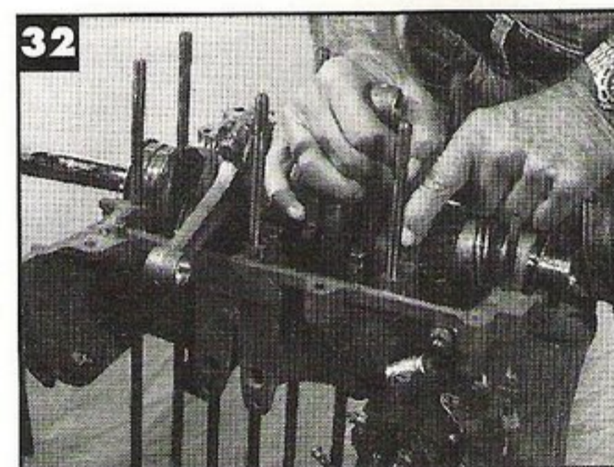
32 - Repeat the process holding the number two rod and engage the other bearings on the dowel pins.
