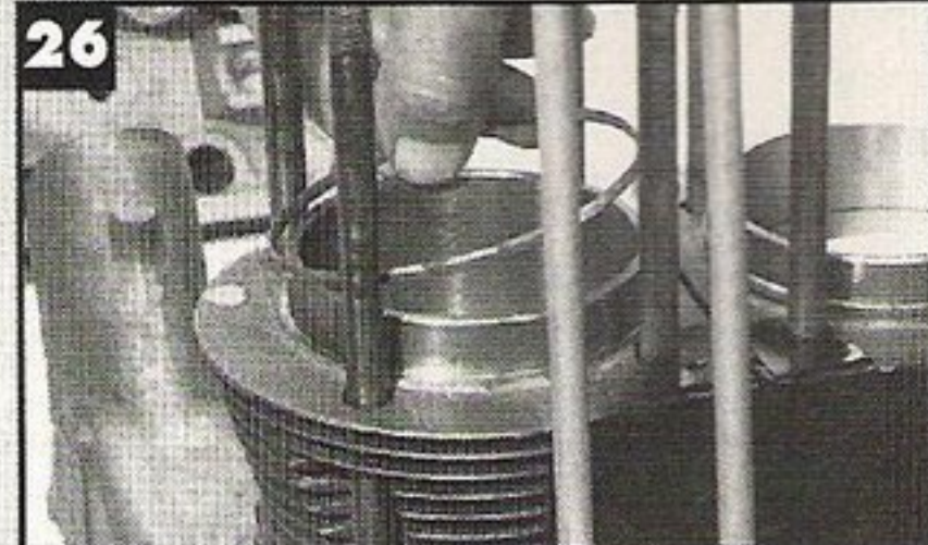
26 - With the pushrods in place, install one copper gasket on each cylinder with the split side of the gasket towards the cylinder head.
