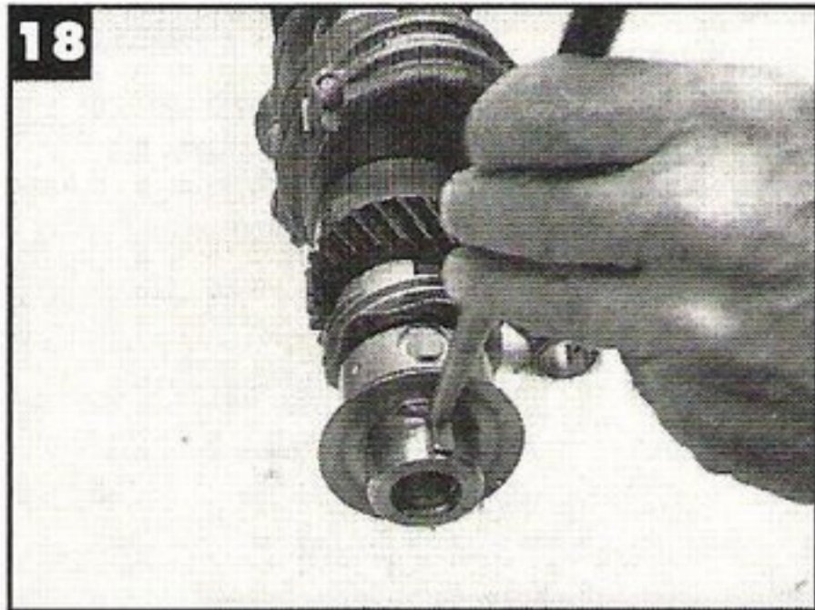
18 - Install the oil slinger ring, ensuring the concave side faces away from the crank. Then include the woodruff key, tapping it in square and firm.
