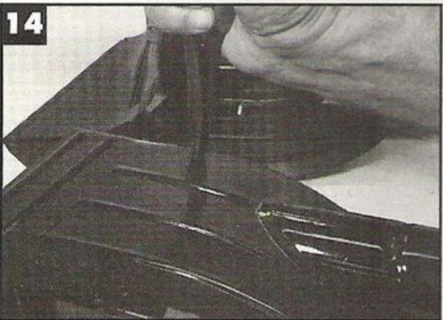
14 - Here is why many tabs may be found broken. They are secured with a slight twist on the outside of the heater channels.
