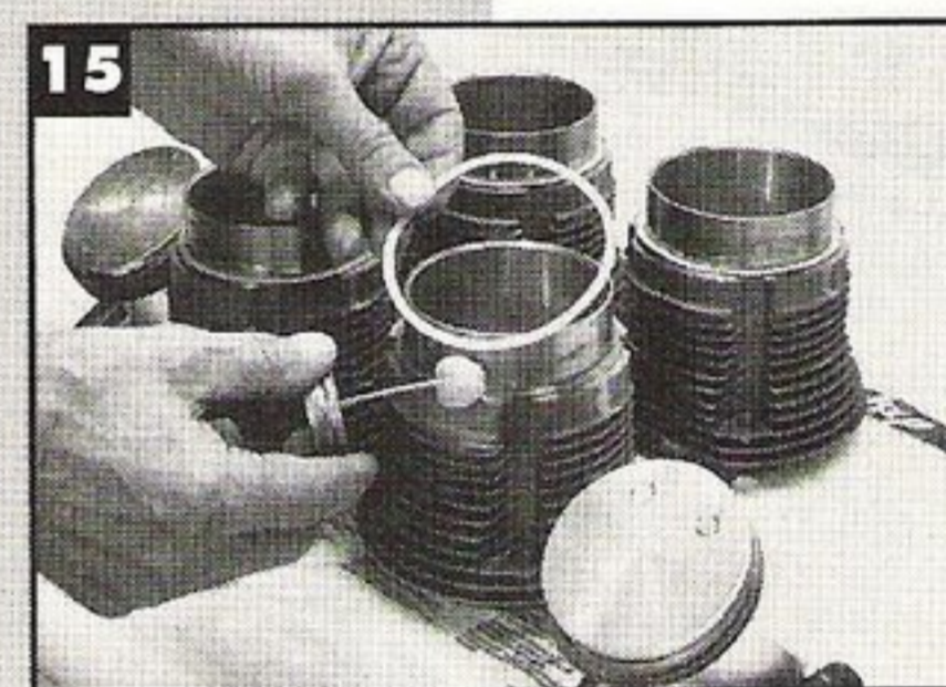
15 - Install the paper gaskets on each cylinder with a thin coat of sealant. This is one of the places on a VW engine that heat-proof real silicone sealant can be used but is normally reserved for stroked engines with metal spacers and no gaskets. It is also difficult to use as it dries fast and thick, requiring a fast assembly of four cylinders pushrod tubes and cylinder heads torqued down before it gets too thick.
