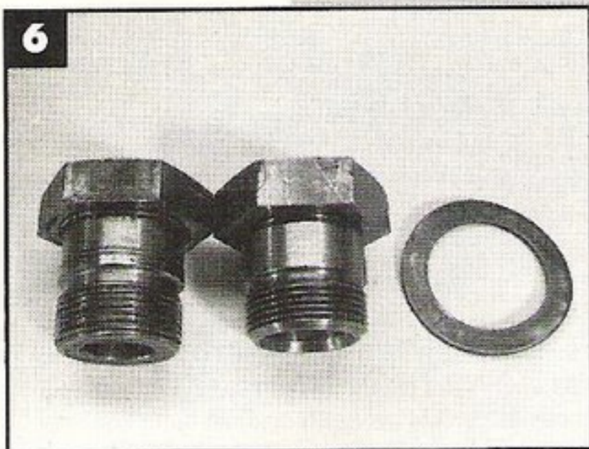
6 - Be sure you have the short gland nut and wavy washer. Install the flywheel on the crank dowel pins and snug up the gland nut.
