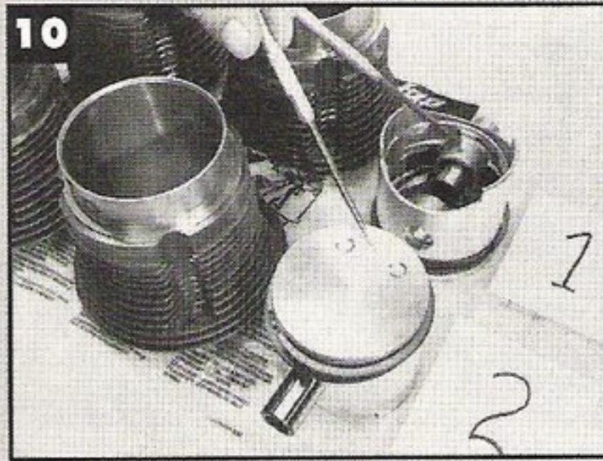
10 - Lay the pistons and cylinders out in order on your bench. Note there is an arrow on top and a bump inside the piston at the wrist pin boss. Both of these indicate that they go towards the flywheel. Ring gaps and side clearance rarely need to be checked when using a new matching set. If you plan on re-ringing the old pistons and honing the cylinders, the ring gaps are .012 to .017 inches on all rings. On the compression ring the side clearance is .0014 to .0022 inches with a wear limit of .008 inches.
