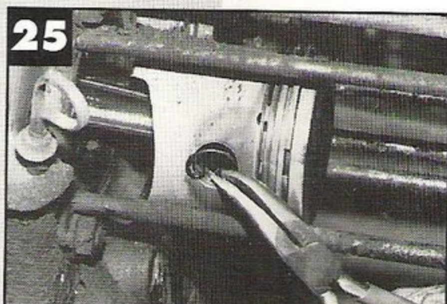
25 - Remove the wrist pin circlips. I have modified my right-angle needle-nose pliers with grooves filed in the jaws.
