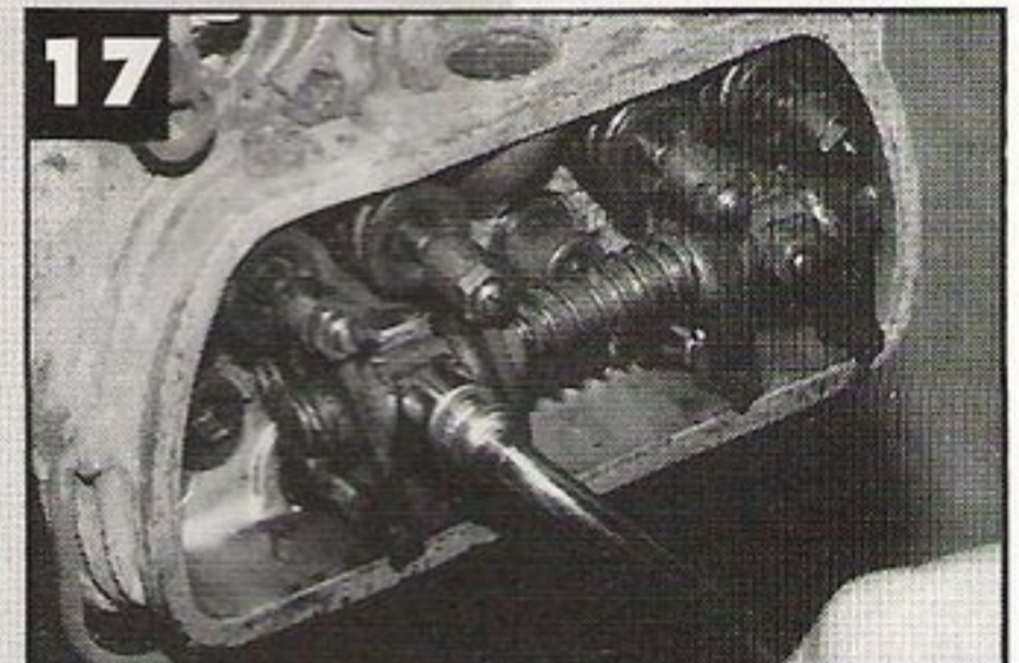
17 - Unbolt the rocker arm shaft. Note the rocker shafts mount differently than later engines; the casting in the head is a half circle and has a curved metal cap on top.
