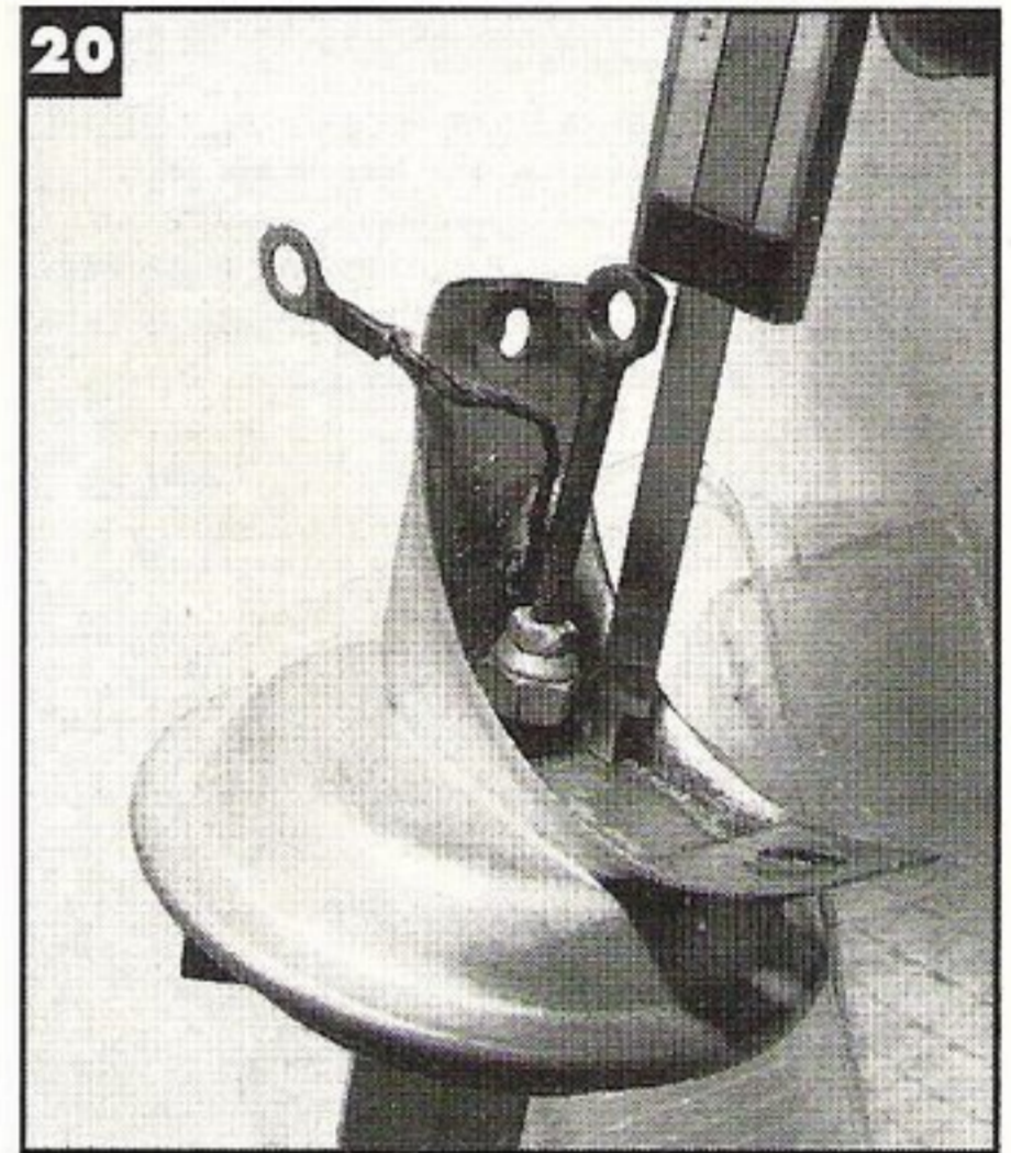
20 - Here is the vacuum advance unit from the VJUR4BR8 distributor, which if functioning correctly will give better gas mileage than a centrifugal-only distributor. Distributors in the VJU4BR8 range also incorporate centrifugal weights and work in conjunction with the vacuum advance to accommodate varying engine load. To correctly adjust the amount of vacuum advance, turn the threaded rod until it measures 1.709 inches plus or minus .008 inches to the vacuum chamber assembly housing. Shown here is a large adjusting nut and small jam nut. Loosen the jam nut and turn the large nut until it measures .138 inches plus or minus .006 inches to the vacuum chamber housing and tighten the jam nut. The long hex-shaped section and nut on the outside of the canister houses an adjustable spring for the diaphragm, which is set at the factory with special tools. No attempt should be made to adjust it.
