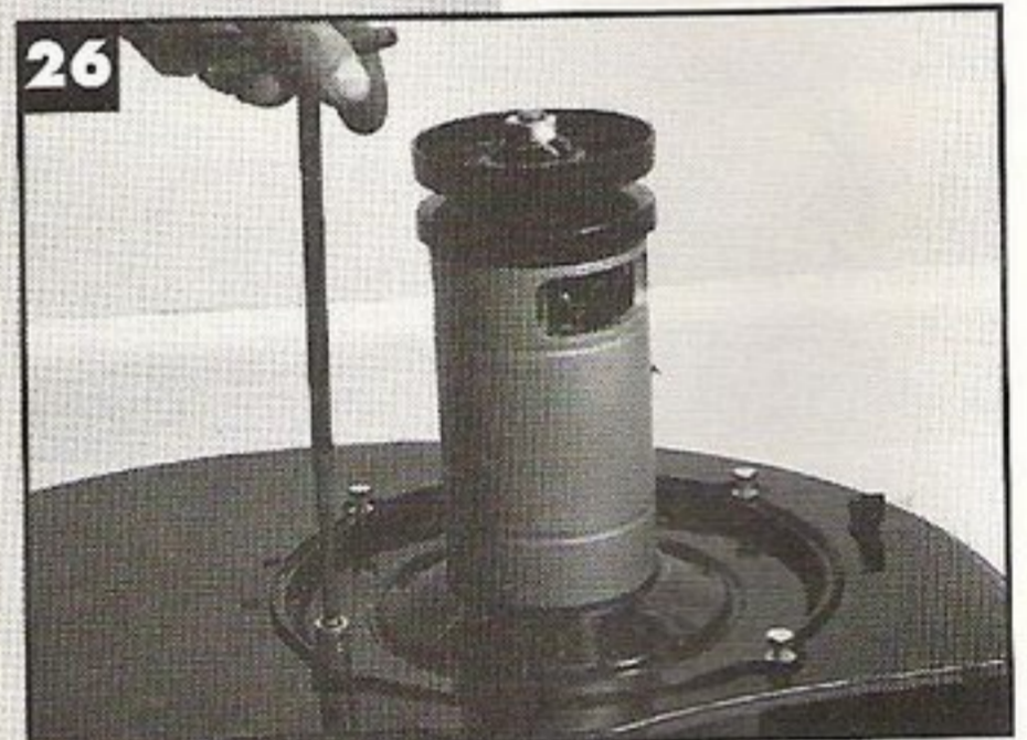
26 - Place the fan in the fan shroud and tighten the four bolts with a 10mm socket. Do not use sheet metal screws here as usually they won't be tight enough and will vibrate loose.
