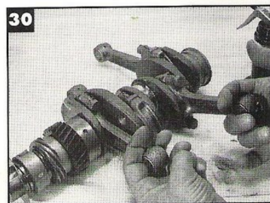
30 - With the distributor in place and rotor pointing to the number one position notch on the rim, pick up the crank as shown by number one and two connecting rods.
